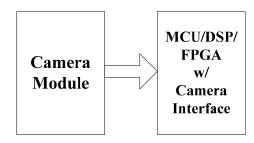
For the host that doesn't have a dedicate camera interface, additional hardware is needed. User need to buffer a entire frame before read them out with low speed MCUs. For example ArduCAM shield is a additional hardware that can be connected to Arduino UNO/Mega board, user can take a photo or something like that easily. The following diagram show the system without dedicate camera interface.
