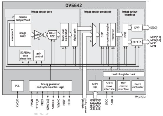
Note: OV5642 camera module only support DVP interface, it doesn't support MIPI interface.
