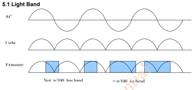
The strength of office light is not even. It changes with AC frequency. For example, if the AC frequency is 50Hz, the light changes strength at 100hz.
